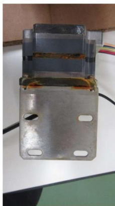
Photo 2: Rust in the Y Motor
